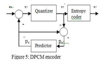
DPCM encoder is shown in figure 5, it is the combination of quantizer, entropy enceoder and a predicator.Here  $p_S$  is the current sample and  $^p_S$  is predicted value,  $^p_S$  is formed using prediction factors and previous samples, for this linear prediction is used, thus predicted value can be given as a weighed linear combination of \_m' previous samples using  $x_i$ , weighting factors:
