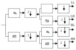
Fig. 2: One filter stage in 2-Dimesional DWT
