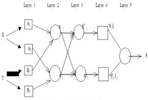
Figure 6: Two level ANFIS structure
